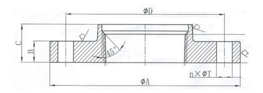
6" Ductile Iron Threaded Flanges with 6 Holes for Ductile Iron Pipe ANSI / AWWA C115/A21.15 Ref: DPF066H
